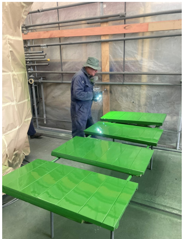
Top left: Brian and Mike start out on the masking . Top Right: Primer has been sprayed on and preparation for the next layer of masking. Mid Left: The black has been sprayed on. Lower Right: Brian inspecting the panels for defects, im sure they passed inspection.. Lower Left: The masking job that certainly deserves some kind of award!
