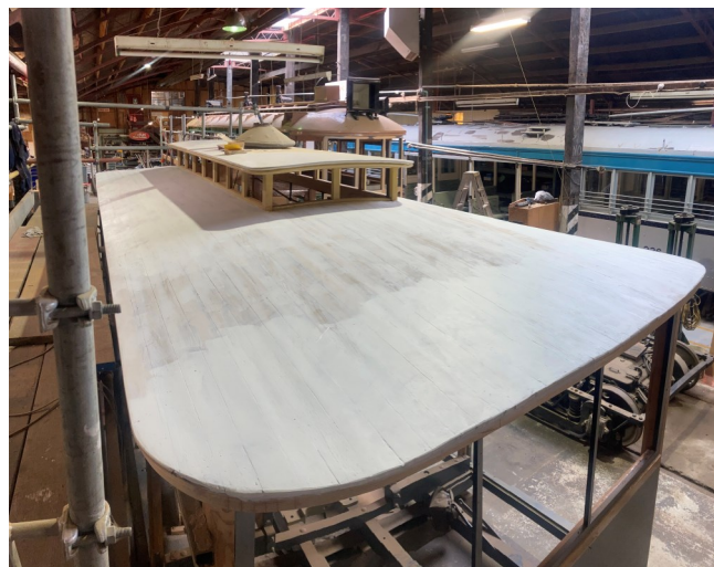
Above: The roof ready for another coat of paint before the Dynel Cloth is fitted.
