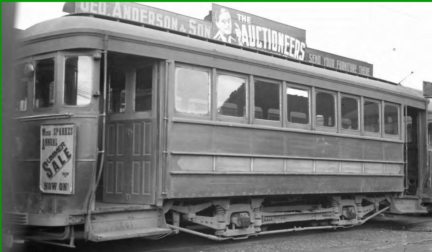
**ABOVE:** 'Standard' trailer 140 stands in the trailer sidings at the Falsgrave Street depot, October 1951. This trailer was one of seventeen (Nos. 126-142) that were equipped with Peckham P21 trucks built by local firm Cooper & Duncan, the others being fitted with Brill 'Radiax E-1' (Nos. 146-149, 201-206). Photo: Graham Stewart.
