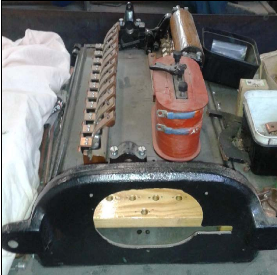
Last (and certainly not least), one of the three partially rebuilt K-10 controllers. We had three incomplete controllers (one as a spare), and the missing parts for each are being made, and the existing parts are being repaired and refurbished. Notice the full set of fingers that have all been manufactured from scratch. One of the interesting items currently being worked on (and not shown) is the manufacture of the new "speed rolls" from cast pieces. I would hope that Jonathan Day can put together a description of this work for Tracts that does it justice.
