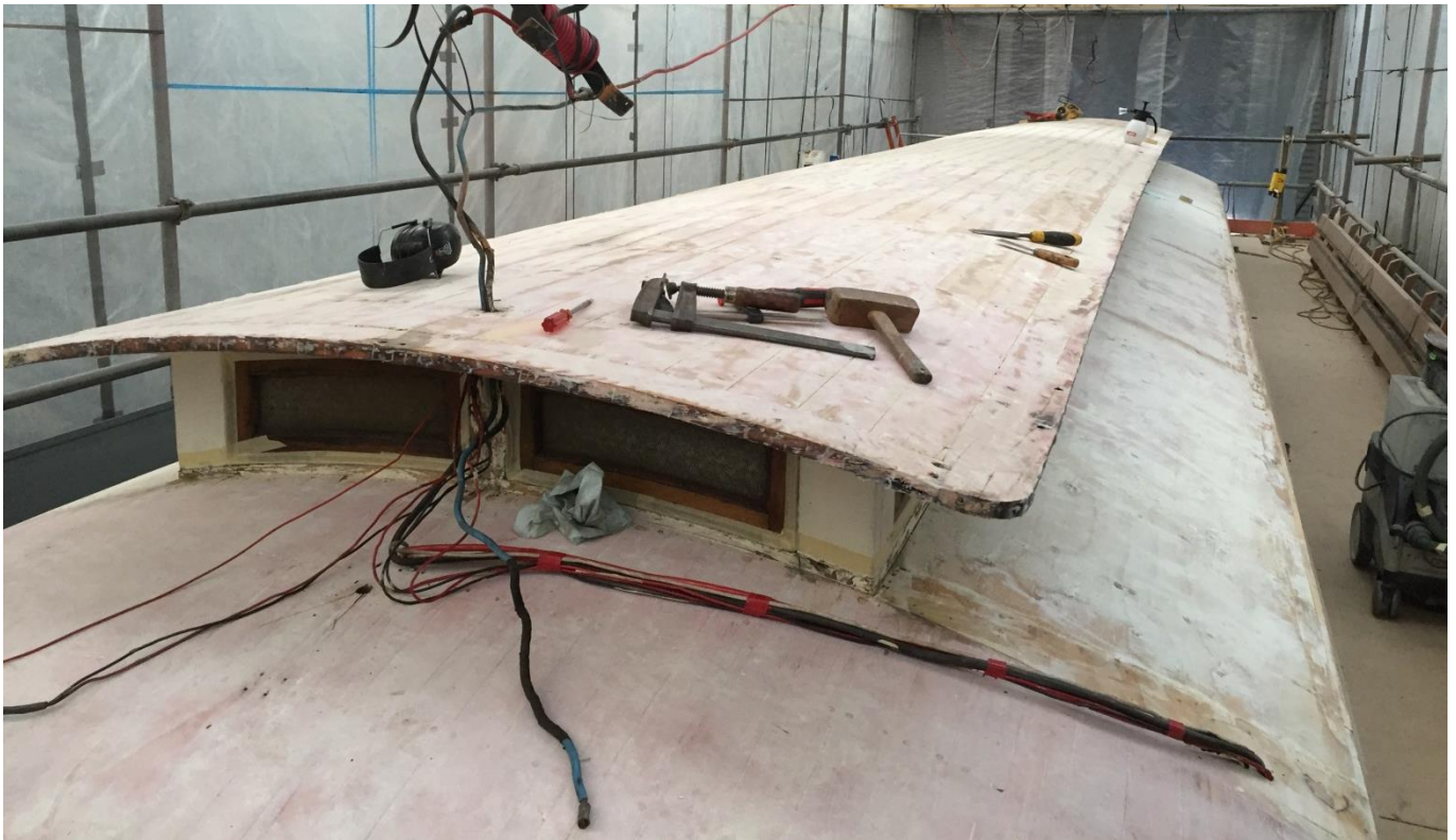
ABOVE: As mentioned by Stephen, Christchurch 152 has returned home to Ferrymead for its roof to be re-canvassed by the Heritage Tramways Trust for the Christchurch Tramway. Currently parked in the paint booth in Tram Barn 3, the tram is shown here with the roof stripped down and ready for the new canvas to be laid. PHOTO: Dave Hinman.
