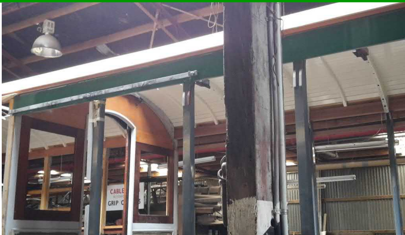
ABOVE: Christchurch 'Hills' car 24, showing the left side letter board painted and in position along with the sliding door and window tracks. Photo: Stephen Taylor.
