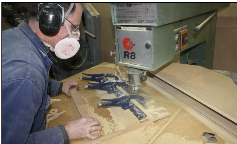
Graeme Richardson cutting new parts for 24's controller as part of an asbestos replacement programme.
