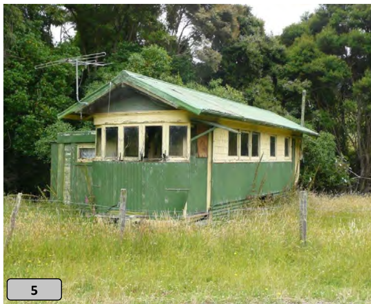
4. The body of No. 126 as seen from the same position, six years earlier in 2010. This side of the body had been little altered from its CTB guise other than the overall roof, porch rooves over the doors and wooden shingles over some of the windows. Photo: Dave Hinman
