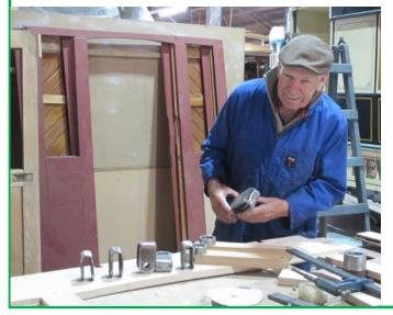
Meanwhile Don Clark (pictured) is making progress welding together all the many clevises required for the moving joints of the wheel brake levers. I have done full sized drawings of the wheel brake blocks. As there are no patterns in the THS storeroom we will now be going to a local pattern maker for a quote. Then we will arrange for the patterns to be cast.
